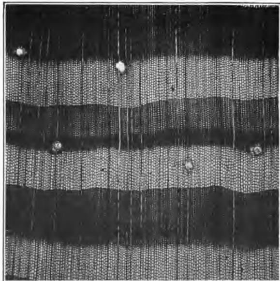
FIG. 2.—LONGLeAF PINE. Cross section magnified 15 diameters.
